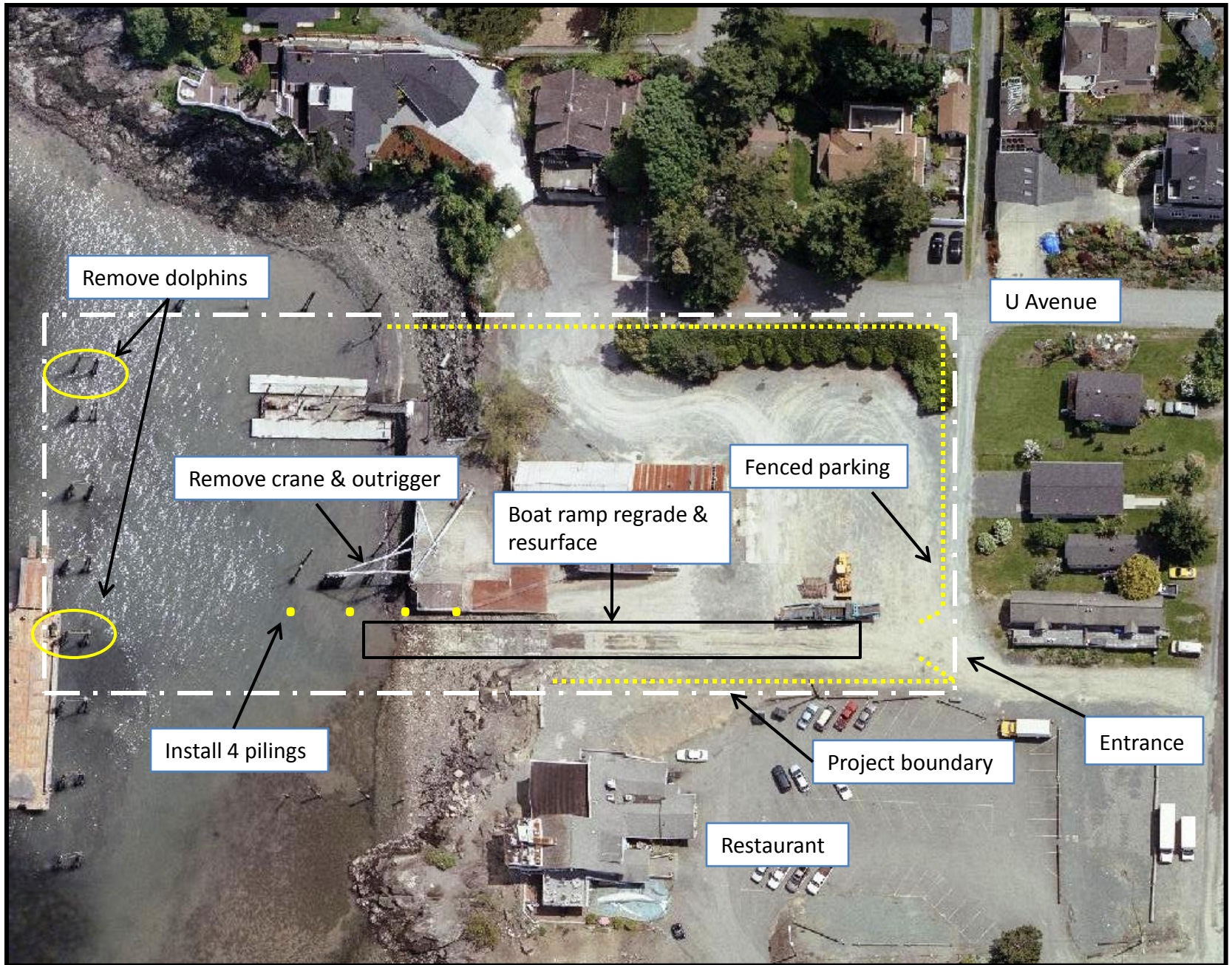
Wyman's Boat Ramp Rehabilitation (not to scale)
