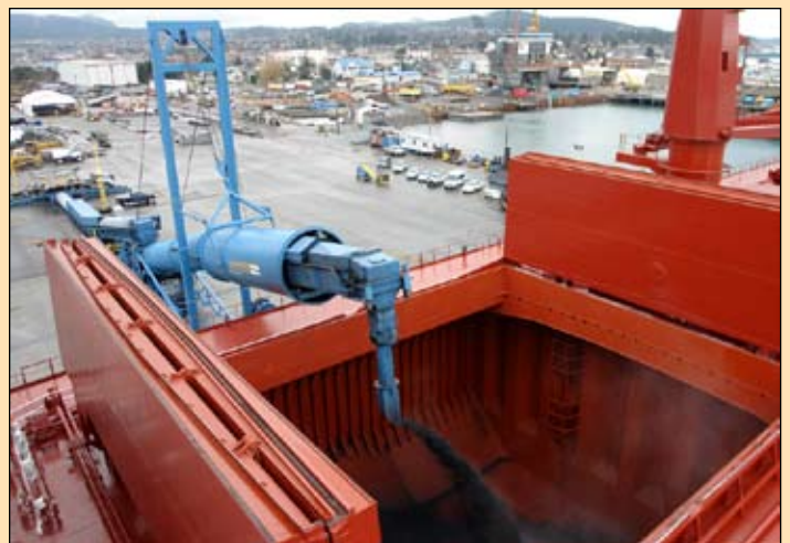
Metropolitan Stevedore Co. facilitates the loading of ships transporting petroleum coke from Anacortes. The blue loader pictured here was engineered specifically to meet a call for a clean, quiet operation at Port Pier 2.
