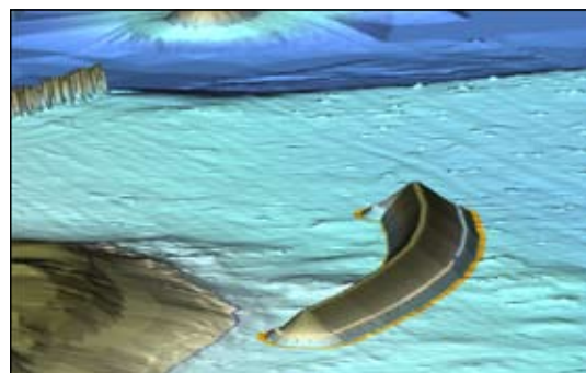
This 3D graphic illustrates Phase One section of a new breakwater to protect the first section of Seafarers' Memorial Park and neighboring bay area. Current pilings (upper left) will be removed.
